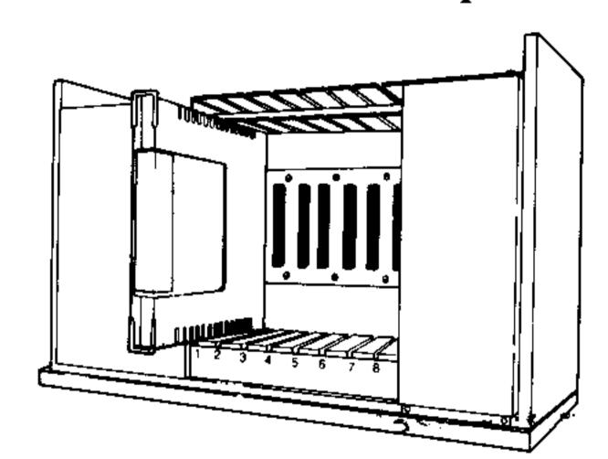
6. Make sure the Memory Expansion Card is inserted in the peripheral system.
